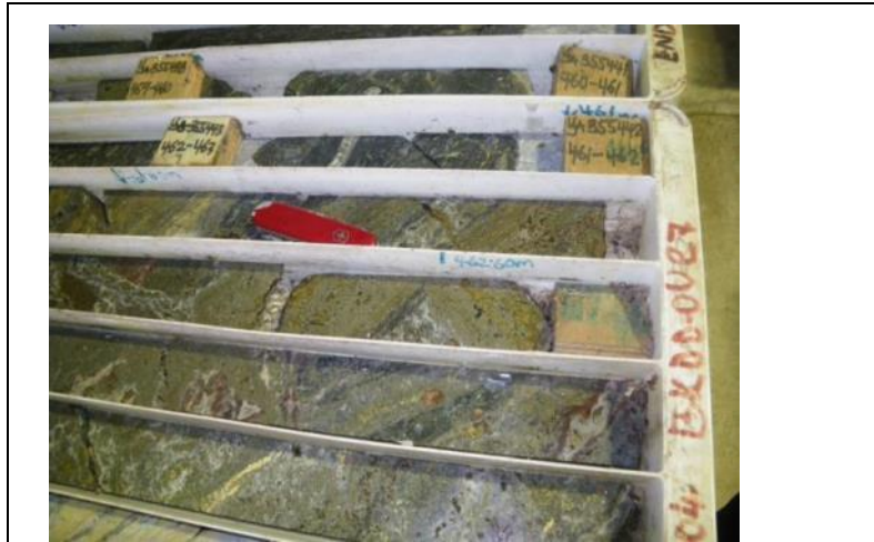
Figure 28: BKDD0027 461.6 to 462.6 m 16.3 g/t Au, 131 g.t Ag and 6.48 g/t Cu
