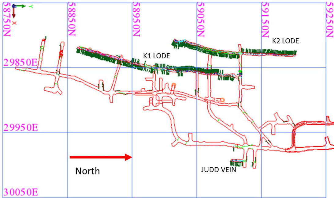
Figure 13: 1185 level plan showing the Judd Vein Drive, K1 and K2 of the Kora North workings
