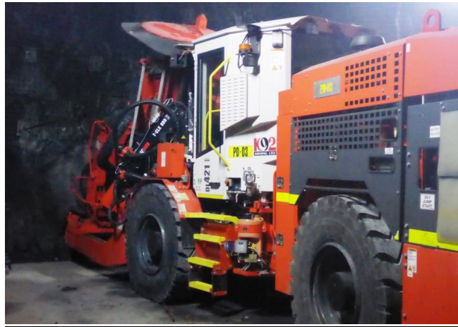
Figure 90. Sandvik DL421 longhole production drill rig
