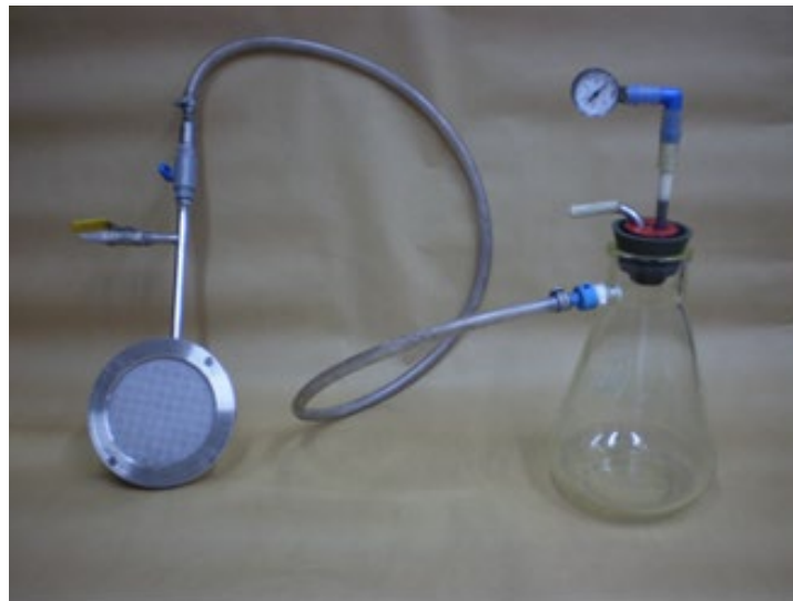
Figure 13.13.5 Photograph Showing the Scanmec Leaf Filter Test
