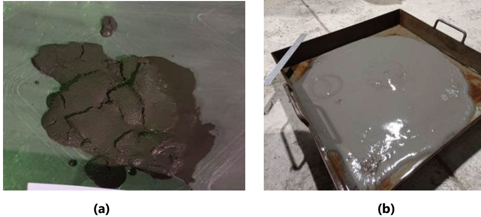
Figure 13.14.15 Kainantu Tailings as (a) Filter Cake and (b) Thickener Underflow at 66% Solids
