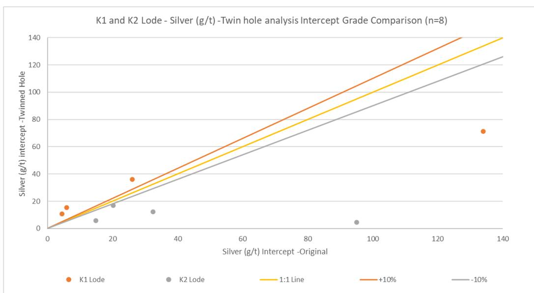
Figure 11-42. K1 and K2 twinned holes original silver versus twinned intercept silver grade.
