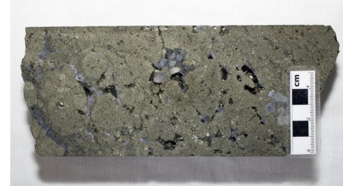
KARDD0002, 148.1m; 71.6 g/t Au, 0.03 % Cu, 15 g/t Ag. Massive, fine-grained pyrite with interstitial saccharoidal quartz.
