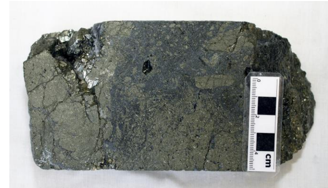
KARDD0002, 223.0m; 6.88 g/t Au, 0.02 % Cu, 6 g/t Ag. Massive pyrite in breccia clasts with rock flour matrix.
