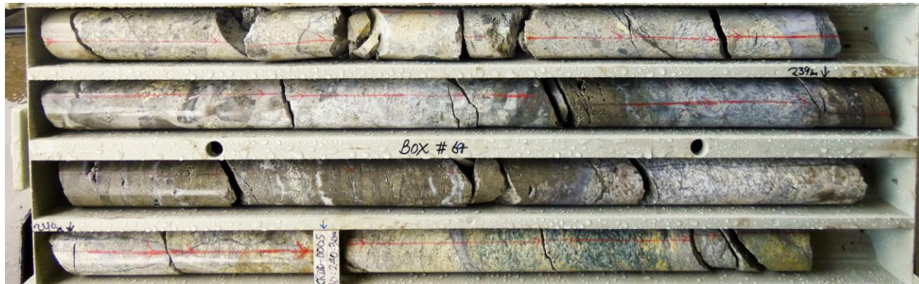
Massive sulphide / quartz vein in sericite altered diorite 2.45m at 39.82 g/t Au, 6 g/t Ag, 0.19% Cu (40.18 g/t AuEq)
