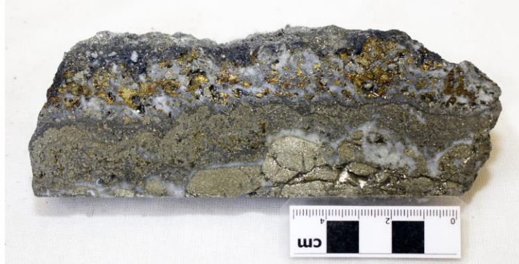
KARDD0002, 103.5m; 7.39 g/t Au, 7.34 % Cu, 73 g/t Ag. Banded semi-massive sulphide (chalcopyrite-pyrite) interspersed with cryptocrystalline quartz.
