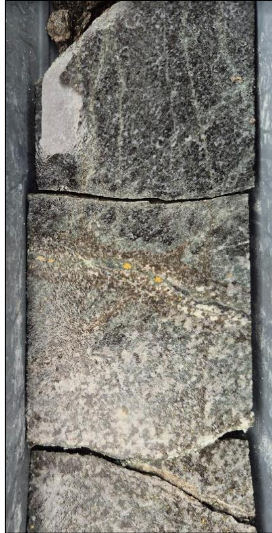
Potassic-altered diorite; cpy, py, trace Bn; from interval 718.5-719.5m grading 0.35% Cu 0.24 g/t Au.
