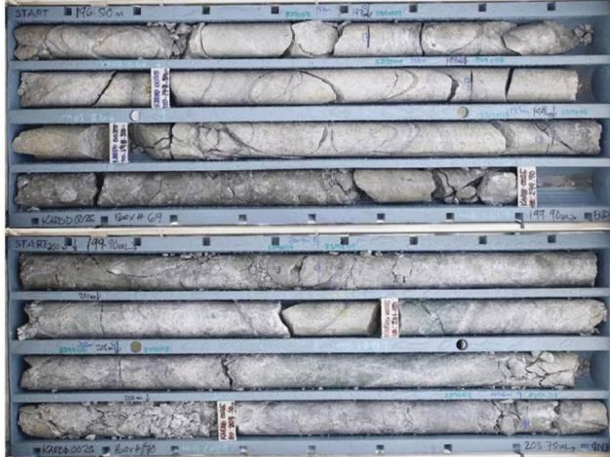
KARDD0025, 196.5 – 211.0m – from 199.0 to 211.0 m is 12.0 m at 11.6 g/t AuEq intersection, within a broader 23.6 m at 6.57 g/t AuEq intersection.
