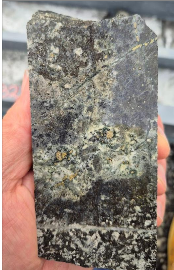
Intrusive breccia; thin sulphide veins (S Veins), disseminated cpy, py, trace bn; from interval 728-729m grading 0.45% Cu 0.21 g/t Au.
