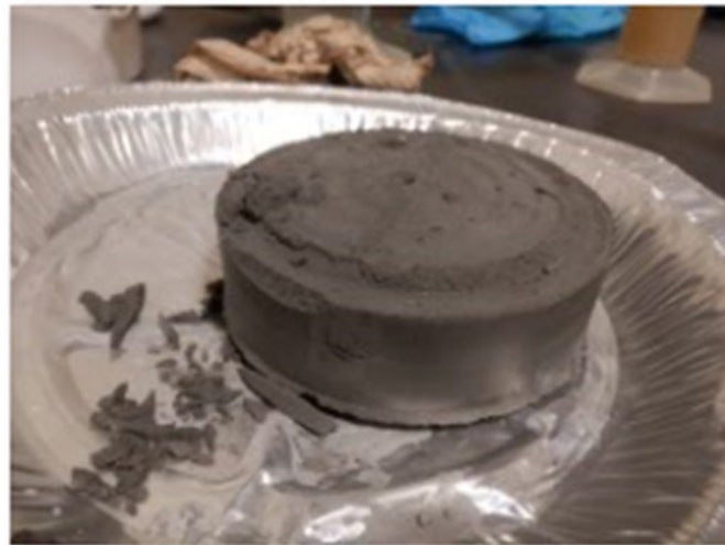
Figure 13-43 Filtered Cake 15-bar Feed, 7-bar Air Blow, 32-mm Chamber, final filtered cake moisture content = 11.8 wt%
