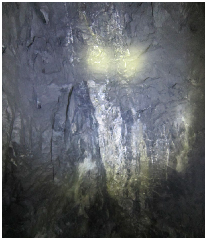
Figure 7-8 J1 Lode showing Quartz-Pyrite Veining (H&SC 2023), (width of image 3 m)
