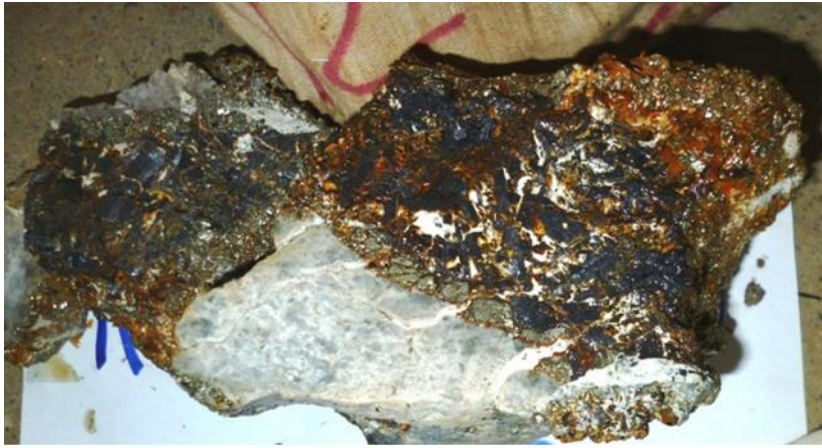
High sulphidation: enargite bearing breccia
